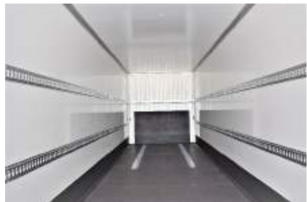
Phenol resin coated plywood
