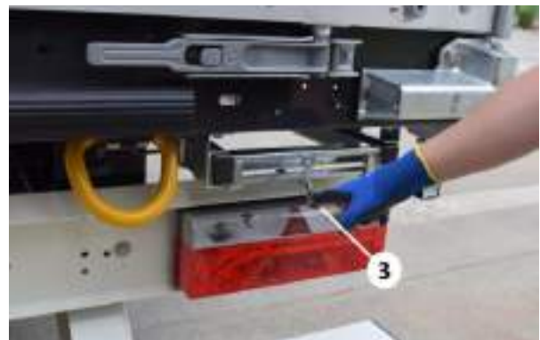
Foldable sliding ladder, removing the pin
