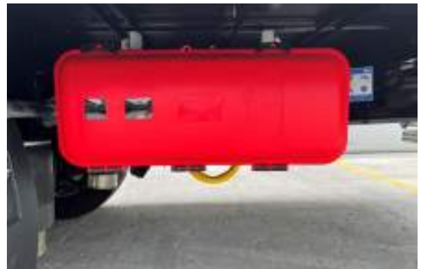
Fire extinguisher box
