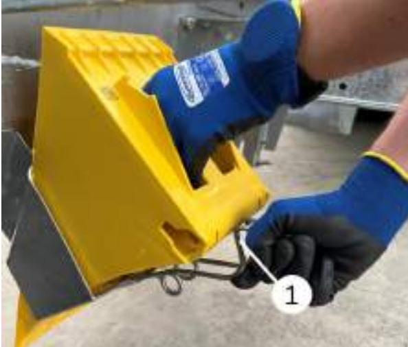
Removing the wheel chock from holders:
