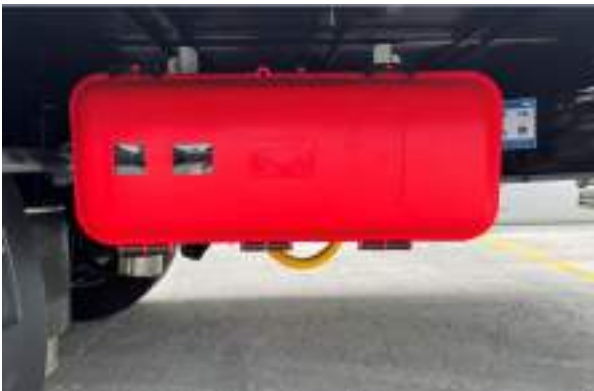
Fire extinguisher cabinet
