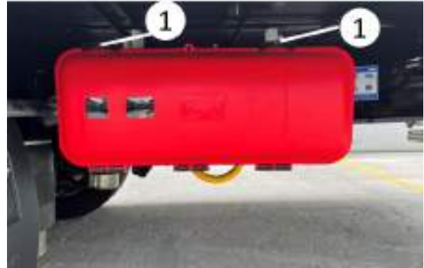
Unlocking The fire extinguisher cabinet
