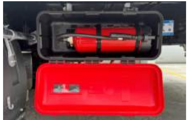
Unlocking The fire extinguisher cabinet
