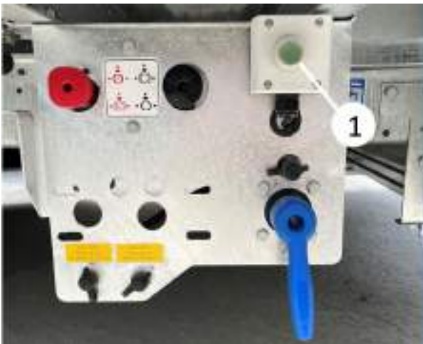
Spring button on the suspension control valve plate
