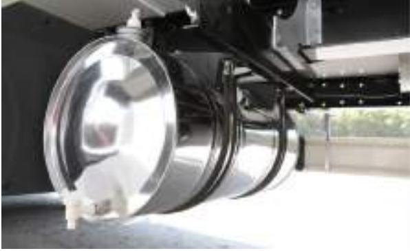
Stainless steel water tank
