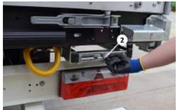
Foldable sliding ladder, removing the pin
